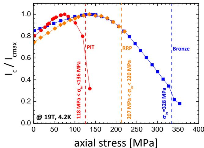
**Figure 2** Critical current versus stress for three Nb<sub>3</sub>Sn wires fabricated by different methods: the irreversible stress limit, indicated by a dashed line, is strongly influenced by the wire fabrication technology.
