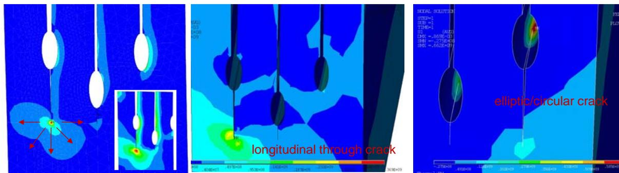
**Figure 5** Local stress concentration and crack propagation for two- and three-dimensional crack propagation analysis using the finite element method. Initial voids are modelled as elliptic holes and the color contours represent the first principal stress for mode I crack.
