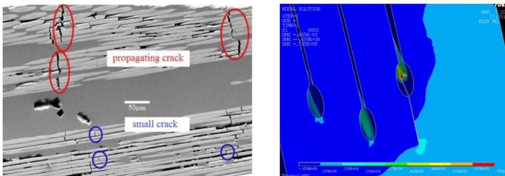
**Figure 3** Micro-cracks observed in the polished longitudinal cross-section of the OST strand after periodic peak bending (left) and modelling of defects with initial crack propagation due to local stress concentration (right).
