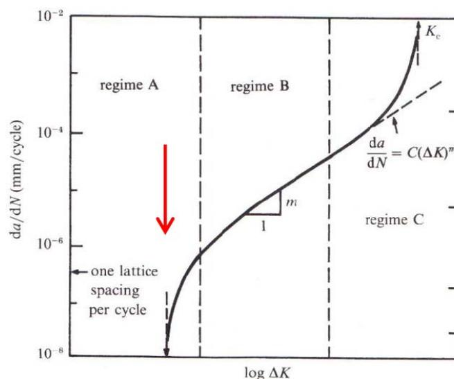
**Figure 4** Schematic illustration of the different regimes of stable fatigue crack propagation. Highlighted in regime A is the crack threshold limit below which crack will not propagate.
