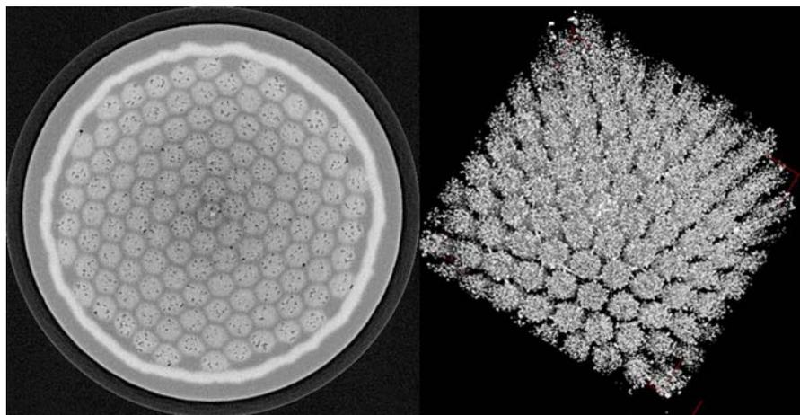
**Figure 1**  $Nb_3Sn$  wire cross section acquired by synchrotron tomography (left) and 3D view of the voids inside the superconducting filaments (right)
